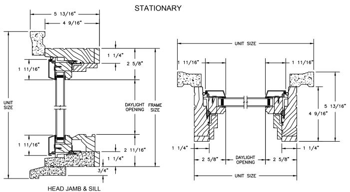
SECTION DETAILS : OPERATING / STATIONARY WITH CONTEMPORARY STOPS SCALE: 3" = 1'-0"
