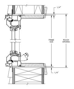
HEAD JAMB & SILL 2 X 6 FRAME WITH SIDING
