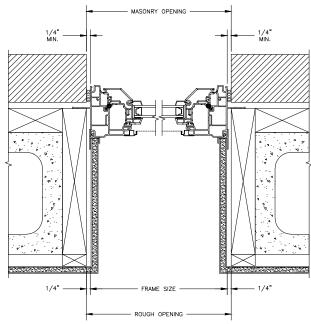
JAMBS 8" CONCRETE BLOCK WALL WITH BRICK VENEER
