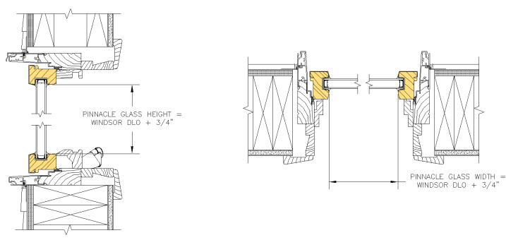
**Note:** Below are the formulas to convert the size of the sash to the correct Pinnacle glass size. The same formula is used for both the width and height.
