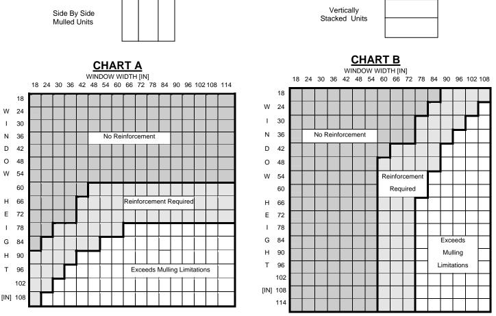
FOLLOWING THESE MULLING GUIDELINES WILL PROVIDE UNITS THAT MEET THE FOLLOWING STRUCTURAL LOADING LIMITATIONS: \* 120 MPH WIND LOAD (80 MPH WITH 1-1/2 SAFETY FACTOR = 120 MPH)
